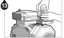
Install the Lubri-Cup EM unit on the lube point.
