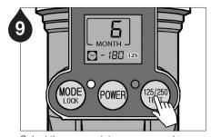
Select the appropriate grease pouch capacity by pressing the 125/250/TEST
