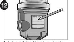
completion date of lube cycle on the lubricator using the label provided in the Service Pack for maintenance purposes.
