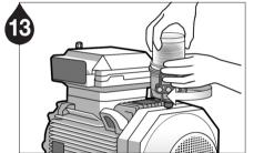
When the selected dispensing period has completed, replace the unit with the Service Pack according to step #3~7.
