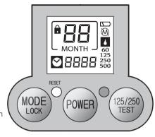
Reset the unit when the unit malfunctions and/or after changing the Service Pack
